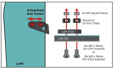
Attach both left Fixie Clips on your left ski using 2x M5x16mm or 2x M5x18mm screws (depending on your board thickness) with 2x M5 square nuts placed in to the nut traps on each. Do not tighten these screws, keep them loose allowing the clip to move side to
