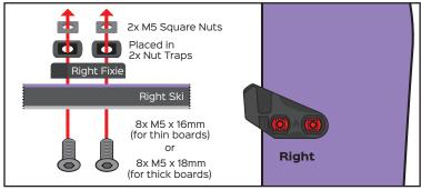
With your board halves apart, securely tighten both right Fixie Clips on your right ski using 2x M5x16mm or 2x M5x18mm screws (depending on your board thickness) with 2x square nuts placed in to the nut traps on the right ski for each clip.
