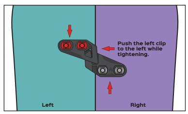
Connect your two splitboard halves while the left clips remain loose. Once together push the middle seam together by either attaching your bindings into ride mode or pushing the board halves together manually. Push the left clip to the left while tightening the left clip screws.
