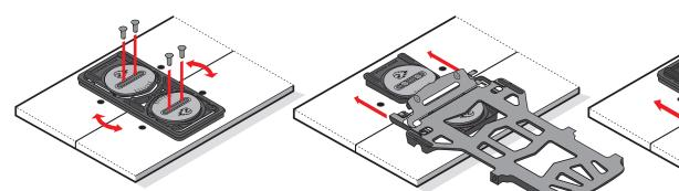
Insert two M6 screws through each disk into the inserts in the board. Tighten a few turns with a screwdriver and then rotate pucks to preferred angle.
