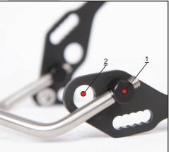
Unscrew the side plates from the bail. Move the bail lugs to hole 1, and reattach the bails, making sure they are threaded completely through the lug.
