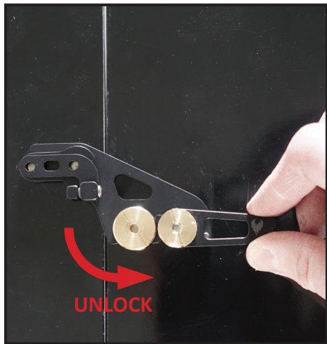
Unlock by rotating the lever counter clockwise.
