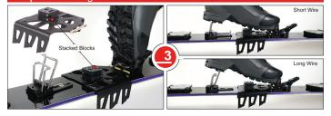
3. As the slope steepens, use the climbing wires together with the climbing blocks on the crampon. The climbing blocks push the crampon teeth into the snow, maintaining traction when the wires are used. Climbing blocks flip up to the stacked position for use with both short and tall wire heights. Forward stride releases boot pressure allowing the crampon to glide freely over the snow.
