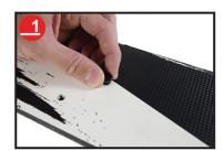
Start by tightening in the center screw into the forward most touring insert, by hand.
