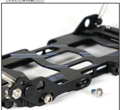
To change bail holes, start by unscrewing the hex screws in the side plates.
