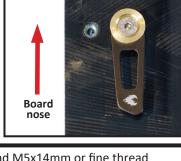
2. Using the flathead coarse thread M5x14mm or fine thread M5x13mm screws install both levers on the right side of your splitboard using the insert farthest from the board inside edge. Tighten. These screws should be tight enough that the levers can be turned easily but have enough friction to stay in place. Rotate the lever toward the tail of your board, out of the way of the remaining insert for Step 3.
