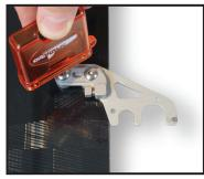
4. Using the buttonhead coarse thread M5x14mm or fine thread M5x13mm screws install both crossbars onto the left side of your splitboard. These screws should be tight enough that the crossbar can be turned and stowed in tour mode with enough friction to stay in place. They should also be loose enough that the crossbar can be moved from ride to tour mode. The tightness of the crossbar is rider preference.
