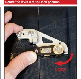
Lever too tight or too loose? Loosen the crossbar mounting screws 1/2 turn then adjust the set screw in the crossbar 1/4 turn at a time to fine tune clamping tension. Once satisfied tighten the crossbar mounting screws.
