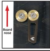
3. Using the flathead coarse thread M5x12mm or fine thread M5x11mm screws install both shear bushings on the right side of your splitboard using the insert closest to the board inside edge. Tighten.
