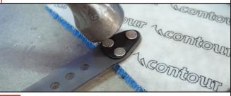
10. Thread the stretcher through the clip as shown in the photo below. Note that there is a right and a left clip, be sure you use the proper clip. Place the clip about halfway down the length of the stretcher and pull hard on both ends to lock the tabs into the holes in the stretcher.
