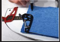
3. Using scissors or a utility knife, trim the skin along the traced line (be careful not to cut the tail stretcher!)
