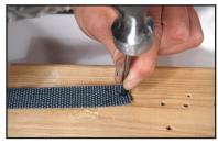
B. Hammer the nail just through the webbing at the three dots using a wood block as a backer. Be sure to push the nail all the way through the holes by hand to ensure the correct hole size.
