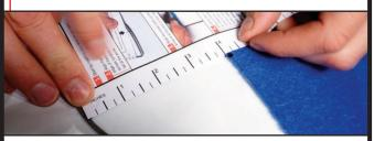
5. Lay the stretcher on the skin with 1" (2.5cm) of overlap. Align the inside edge of the stretcher with the mark made during step 3. Using a marker, make three dots on your skin through the three holes in the end of the stretcher.
