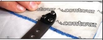
9. Place the skin on a hard durable surface (i.e. concrete or pavement). **DO NOT** use a surface that could be damaged by hammering. (i.e. tile or wood flooring). Using a hammer, lightly tap 5-10 times straight down onto each rivet. Non-vertical taps will lead to crooked rivets (we gave you one extra rivet set just in case). Flip the skin over and repeat.
