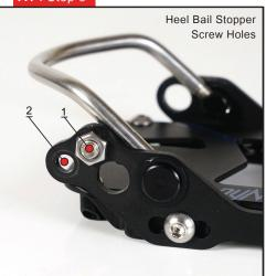
Reattach the bail assembly to the baseplates in the position recommended in steps A2 & A3. Move the stopper screw on the side plate to hole 1.
