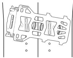
8. Remove the alignment tool and slide your bindings onto the pucks and secure with snap ramp or pin. If you're unable to secure your bindings loosen the screws, nudge in the toeside puck and retighten the screws.
