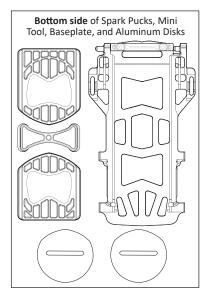
1. Insert an aluminum center disk into each puck with the degree indicators pointing toward the pointed end of the puck.
