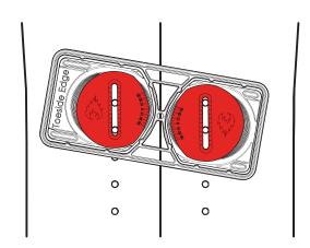
5. Drop an aluminum center disk into each of the pucks. Degree indicator marks should point toward the center line of the board. Rotate so you can see the board inserts through the slot in the disk.
