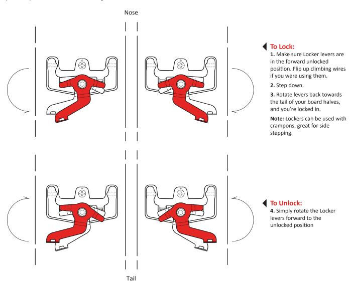
**Note:** If you can't rotate the Locker to the locked position you may need to clear snow off the top of the heel rest or the baseplate where it contacts the heel rest.
