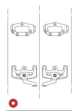
5. Insert the M6-12mm button head screws into the hubs and tighten with the M4 hex key. Tighten the screws so there is sufficient friction to hold the Locker in either the locked or unlocked position.
