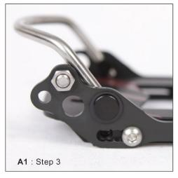
Reattach the bail assembly to the baseplates in the position recommended in steps A2 & A3. Move the stopper screw on the side plate to hold the bail in the upright postion.
