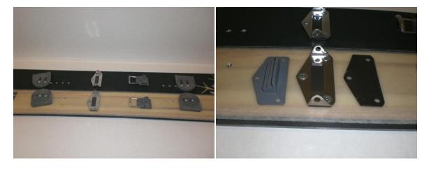
Having the pins insert from the inside in board mode works for most riders. If your pins hit the heel rests because you have a forward angle on your rear foot there are a few options for you.
